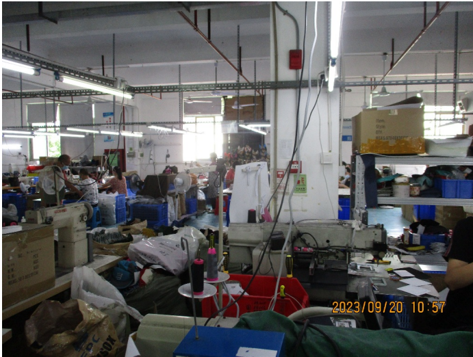
Fire alarm was obstructed by production machines.
